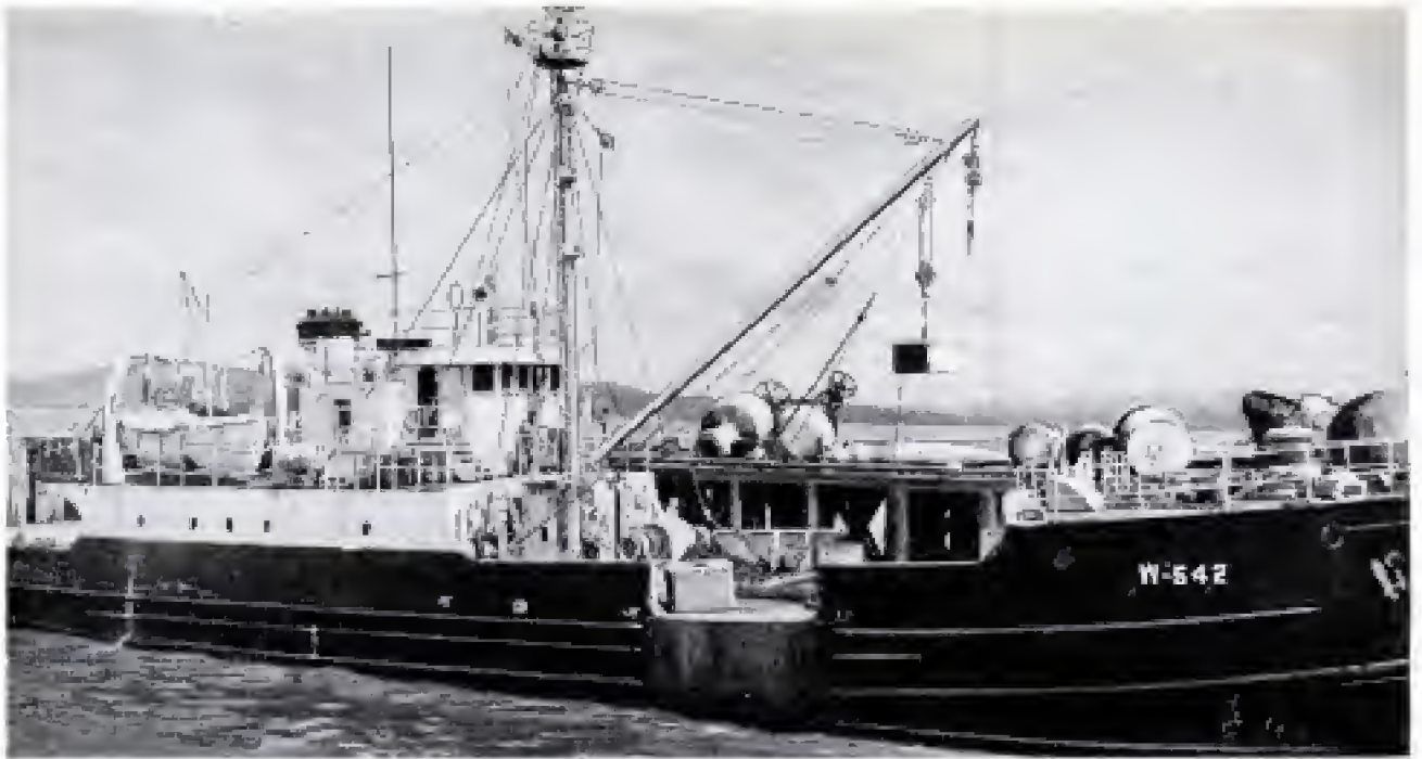
Nine-ton concrete block used in anchoring huge buoys is loaded aboard one of the busy Coast Guard ships
